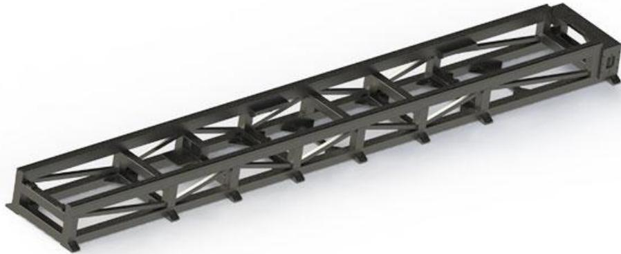
The crossbeam adopts a steel structure welding process, which is formed by precision mechanical processing after overall annealing, reducing weight and improving rigidity. This greatly improves the response speed of the machine tool.
